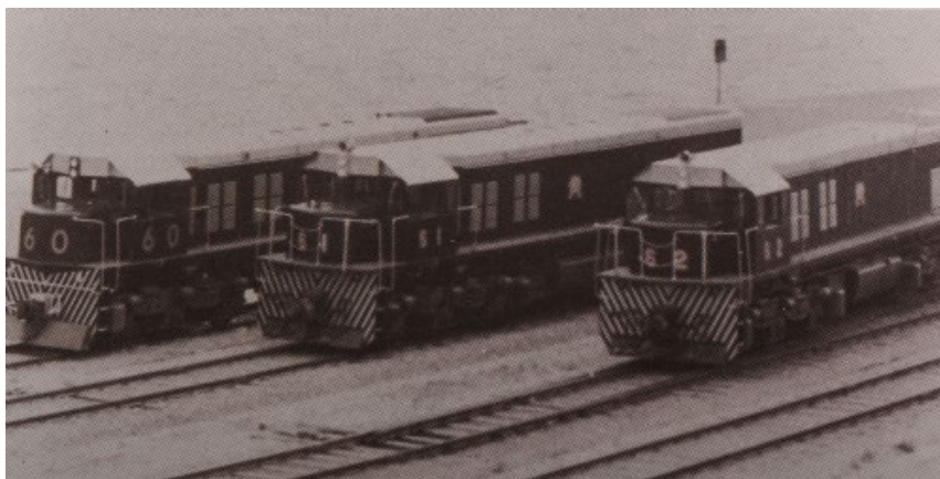
九廣鐵路添置的 60 至 62 號柴油機車，馬力達 2000 匹，將柴油機車車隊的效能進一步提升。 Acquired by the Kowloon-Canton Railway, locomotives Nos. 60 to 62 were equipped with 2,000-horsepower engines which helped increase the efficiency of the diesel locomotive fleet. (香港文化博物館藏品 Collection of the Hong Kong Heritage Museum)
