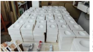
模製鱗片工序相當繁複,而 製作過萬片鱗片亦甚耗時。 The production of over 10,000 scales by slip casting is a complicated and time-consuming process.
